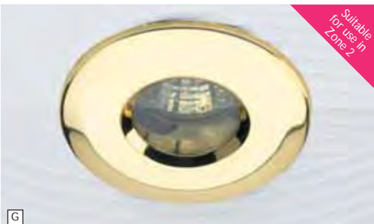
G MR16 Low Voltage IP65 Shower Downlight Cut-out: 75mm. Void depth: 135mm. Rim dia: 87mm. Lamp: 35W MR16 Sealed Dichroic. Quote: MM31131 (White finish) Quote: MM31132 (Polished Brass finish) Quote: MM31129 (Polished Chrome finish) Quote: MM31192 (Brushed Chrome finish) Quote: MM72034 (Gun Metal finish)
