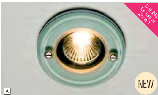
A Mains Voltage GU10 IP65 Glass Shower Downlight Clear flat glass. Cut-out: 70mm. Void depth: 135mm. Rim dia: 100mm. Lamp: 35/50W GU10 aluminium reflector. Quote: MM72117
