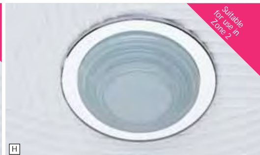
H MR16 Low Voltage IP44 Bathroom Downlight With Opal Glass Cut-out: 75mm. Void depth: 130mm. Rim dia: 96mm. Lamp: 35W MR16 Sealed Dichroic. Quote: MM31162 (Polished Chrome finish)
