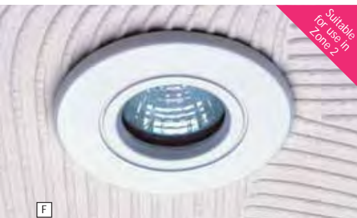
F MR16 Low Voltage IP44 Bathroom Downlight Cut-out: 75mm. Void depth: 130mm. Rim dia: 85mm. Lamp: 35W MR16 Sealed Dichroic. Quote: MM31157 (White finish) Quote: MM31159 (Polished Chrome finish) Quote: MM31191 (Brushed Chrome finish)
