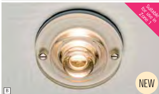
B Mains Voltage GU10 IP65 Glass Shower Downlight Round tiered glass. Cut-out: 70mm. Void depth: 135mm. Rim dia: 100mm. Lamp: 35/50W GU10 aluminium reflector. Quote: MM72118
